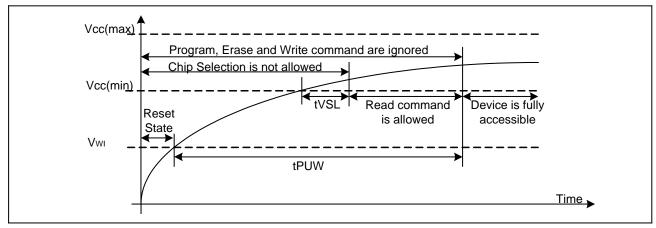
Table3. Power-Up Timing and Write Inhibit Threshold
