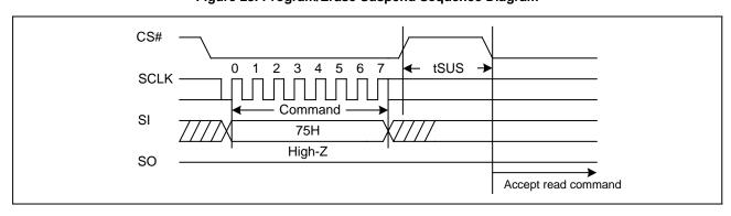
Figure 28. Program/Erase Suspend Sequence Diagram
